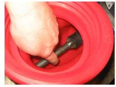
The connecting drive shaft must align with the square receiver on the rigid coupling.
