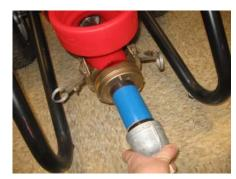
Slide out the stator tube & pump
