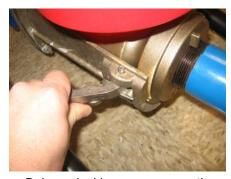
Release locking cam ears on the pump housing base.
