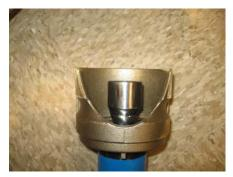
The rotor should stick out approx. 2" as shown. Verify the gasket in the brass retainer stays in place.
