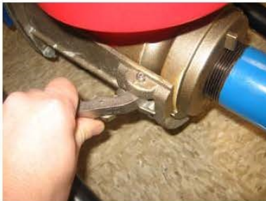
Release locking cam ears on the pump housing base.
