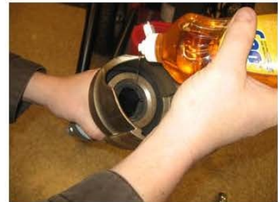
Thoroughly lubricate the inside of the stator tube with liquid dish soap.
