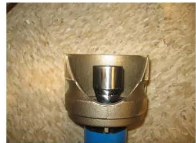
The rotor should stick out approx. 2" as shown. Verify the gasket in the brass retainer stays in place.
