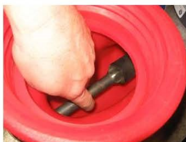
The connecting drive shaft must align with the square receiver on the rigid coupling.
