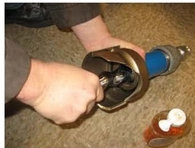
Screw and push the rotor into the stator tube, counter-clockwise.
