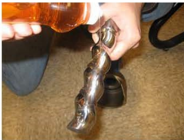
Apply a liberal amount of liquid dish soap to the outside of the rotor.
