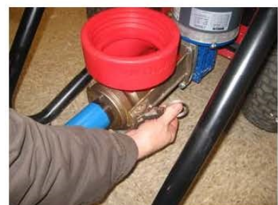
If the rotor is inserted far enough and the connecting drive shaft is aligned, the assembly will slip back position and cam ears will lock back in place.
