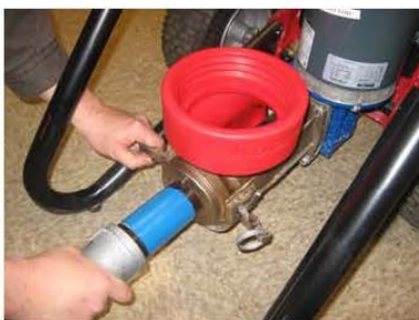
Slide rotor-stator assembly into pump housing base. If it does not go all the way back, check the connecting drive shaft alignment.
