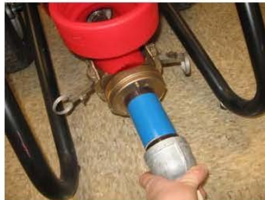
Slide out the stator tube & pump
